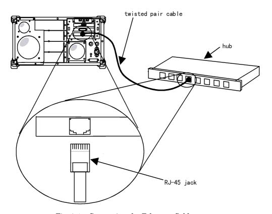
Fig. 2-1 Connecting the Ethernet Cable
